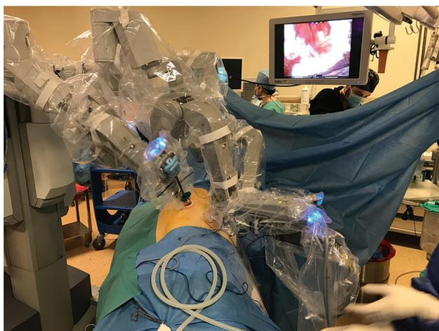
Figure 4: View of the robot after docking on the patient
